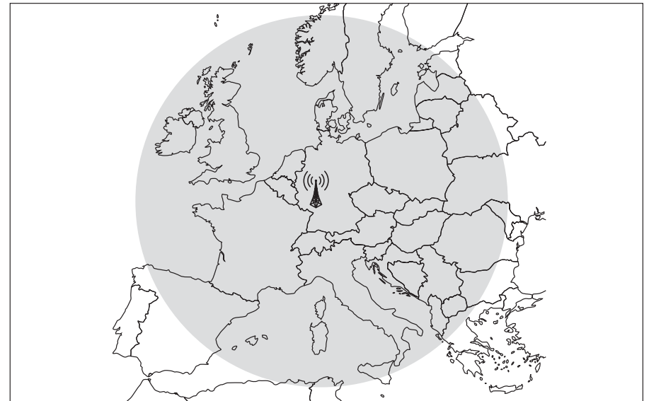
EUR: DCF77 (Germany) Mainflingen: Radius of approximately 1,500 km from the transmitter
